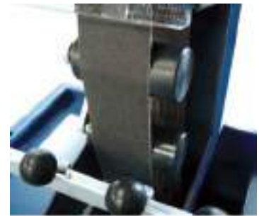
Belt position "straight grinding"
