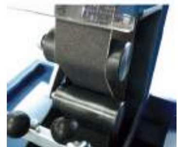
Belt position "upper edge grinding"
