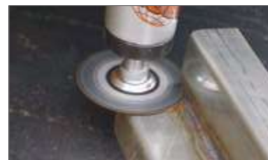
Thin cutting disc Safecut DC: 75x1,0x9,53 A60SX
