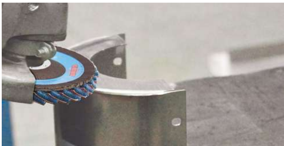
Cleaning and polishing of weldings on stainless steel tubes: before and after.
