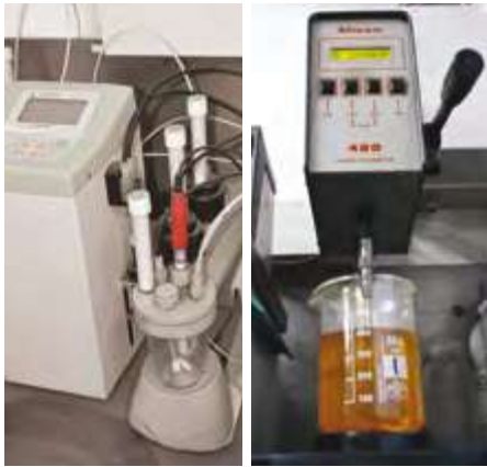
Titration of chemical compounds. Determination of viscosity.
