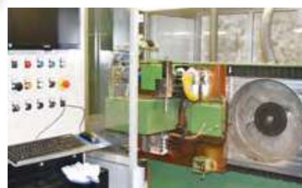
(Pic. 5) Machine for side load test and impact test.
