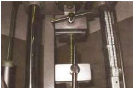
Yarn resistance test of fiberglass reinforcements.
