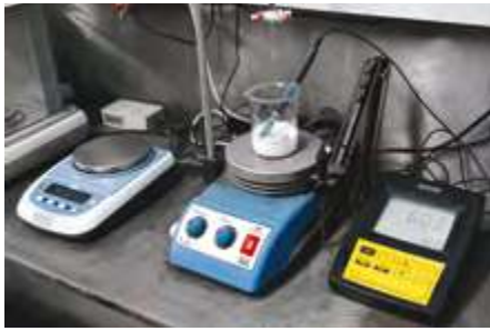
PH metric titration of resin powder.
