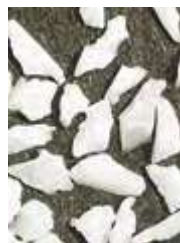
Ceramic grains viewed under a microscope.
