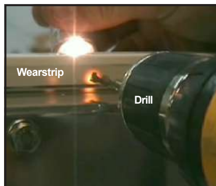
Figure 15: Use light to locate hole; drill hole in wearstrip
