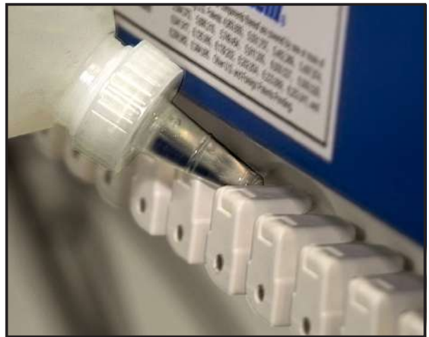
Lubricate the conveyor wearstrip with silicone oil
