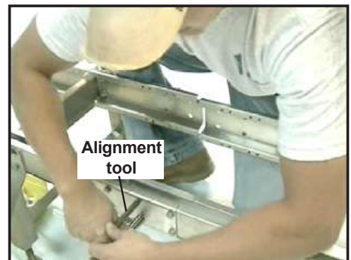
Figure 6: Use alignment tool (in open hole) to draw Bed Sections together
