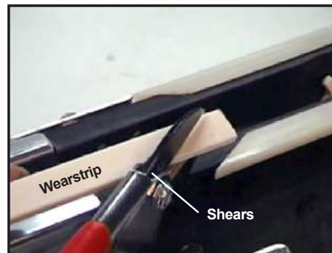
Figure 13: Cut wearstrip at 60° angle
