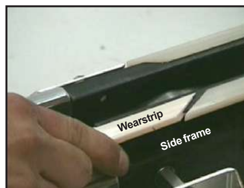
Figure 14: Slide wearstrip into side frame
