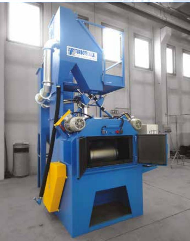
The **GB cylinder blast machines** are designed specifically for treating LPG cylinders, fire extinguishers and cylindrical items in general. The material, which is loaded into the blast chamber horizontally, is made to rotate around its own axis: the blast wheels are positioned to ensure full blast coverage of the cylinder walls and heads. Paint removal, rust removal, descaling, preparation prior to painting for tanks and cylindrical items.
