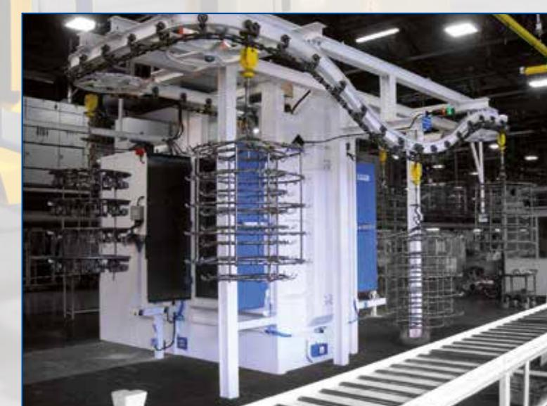
**BETA overhead conveyor blast machines** feature motorized hoists that allow parts to be handled without any weight or size restrictions, making them versatile in terms of their application.
