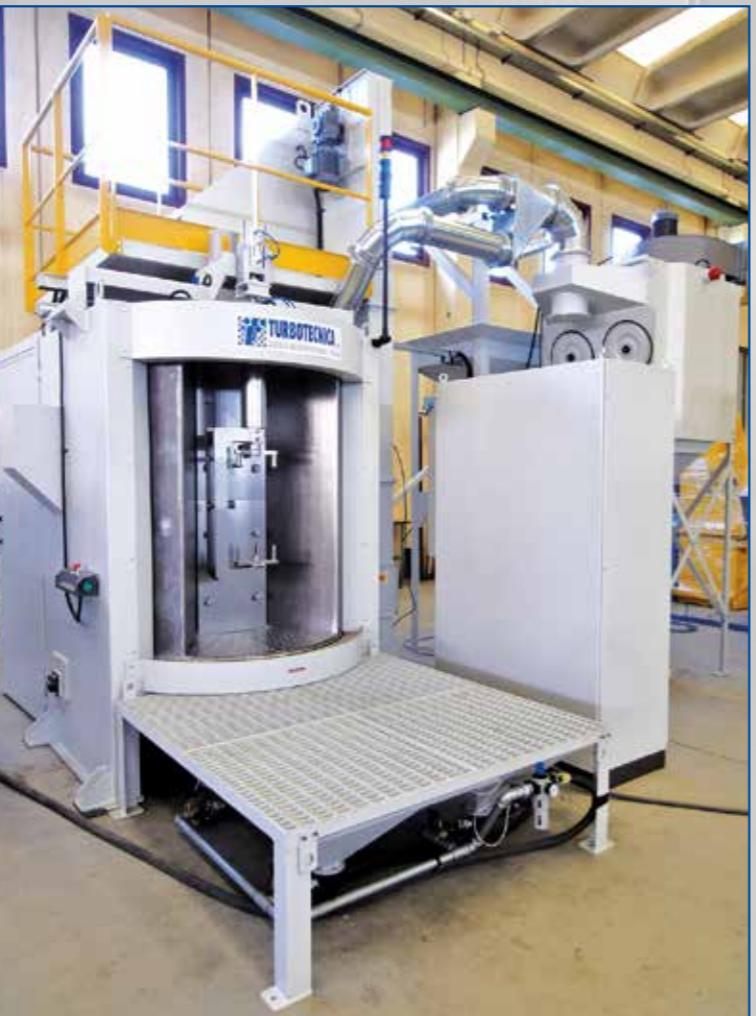
The **TRV vertical rotating table blast machines** are particularly suitable for the surface treatment and deburring of aluminium parts, descaling of forgings and desanding of castings, especially when dealing with workpieces whose shape or size makes them not suitable to tumbling.
