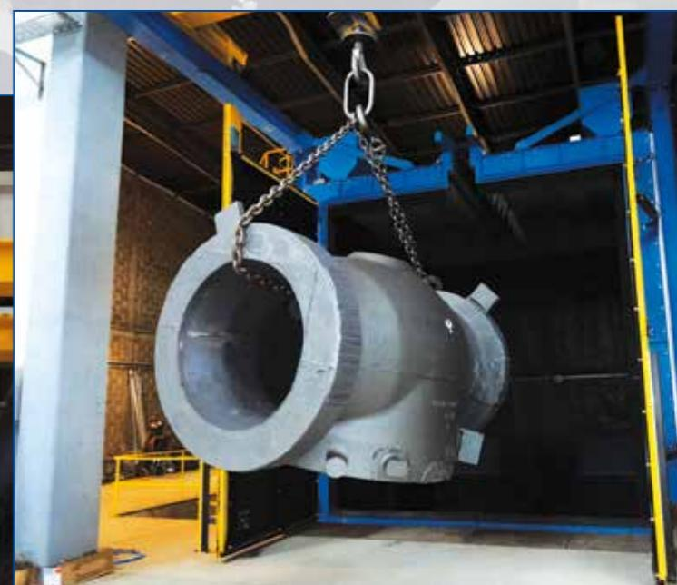
The **TC overhead conveyor blast machine** has been designed to treat medium/large workpieces handled by an overhead conveyor consisting in a monorail, bi-rail or hoist system, or by means of bogies.
