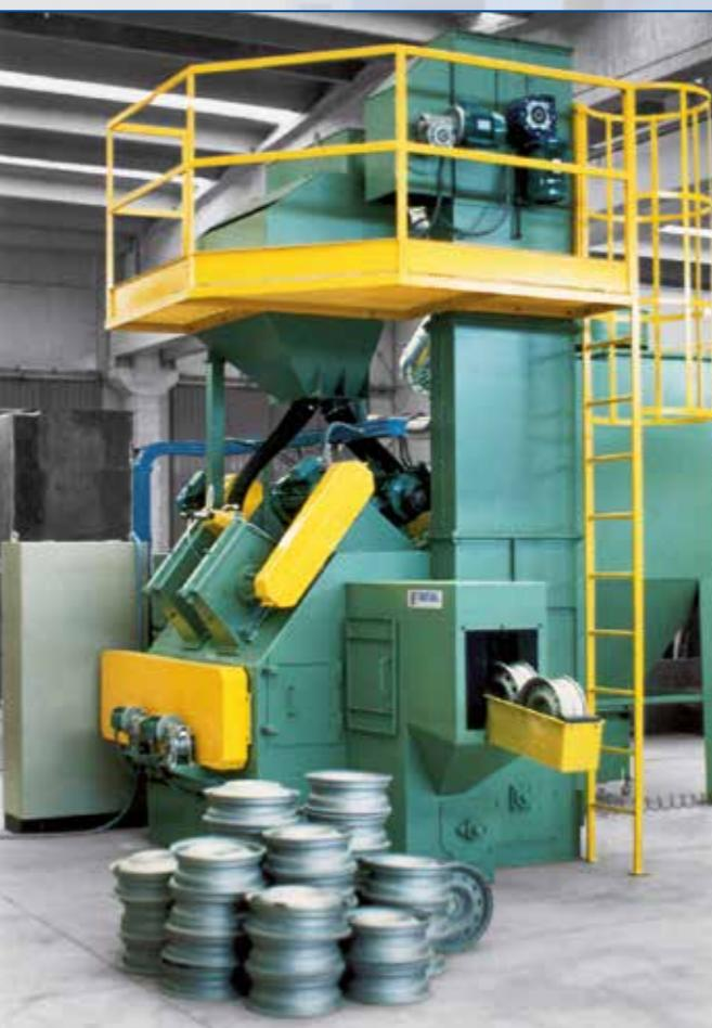
Our **GR wheel blast machines** have been specifically designed to treat steel and light alloy wheels. Paint removal, reconditioning, rust removal, descaling, preparation prior to painting, deburring.
