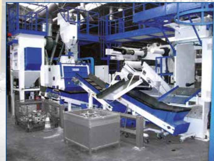
The **TB G** rubber belt shot blasting systems are used for the treatment of high volume bulk parts, which can be loaded into the machine either manually or automatically by means of a hydraulic bucket.
