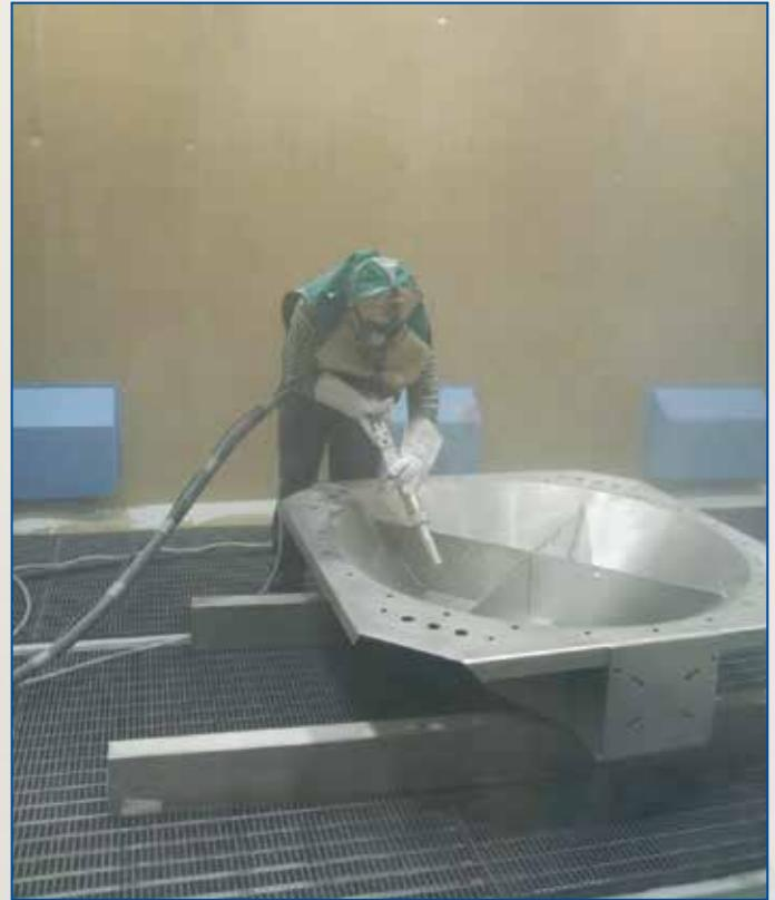
Our professional blast rooms are designed according to the customer's needs and quick and convenient to install with no need to build foundations. *Turbotecnica* blast rooms come with lighting and ventilation systems and protective accessories to ensure the utmost operator safety and the respect of the international standards.
